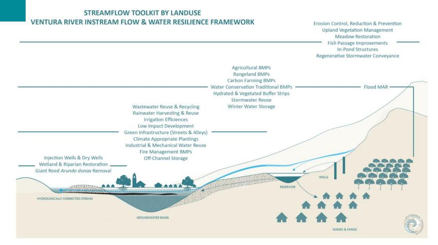
Fig.1: Streamflow toolkit by land-use shows what project types can be used throughout landscapes at a watershed scale to benefit and enhance stream flow for the Ventura River Instream Flow Enhancement and Water Resilience Framework.
