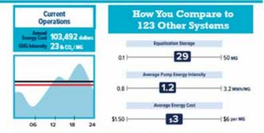
This report presents the results of our simulation for your system and estimates how you could use the energy demand management software (EDMS) to operationalize your system's pumping energy demand flexibility: using available water storage capacity to shift the timing of pump energy use, while maintaining reliable pressure to your customers, in order to take advantage of lower energy costs and reduce greenhouse and entissions.
