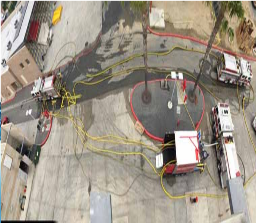
Multiple Engine Pumping Evolution
