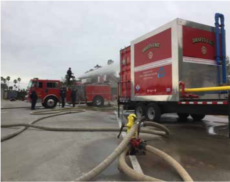
Portable Hydrant & Deck Monitor
