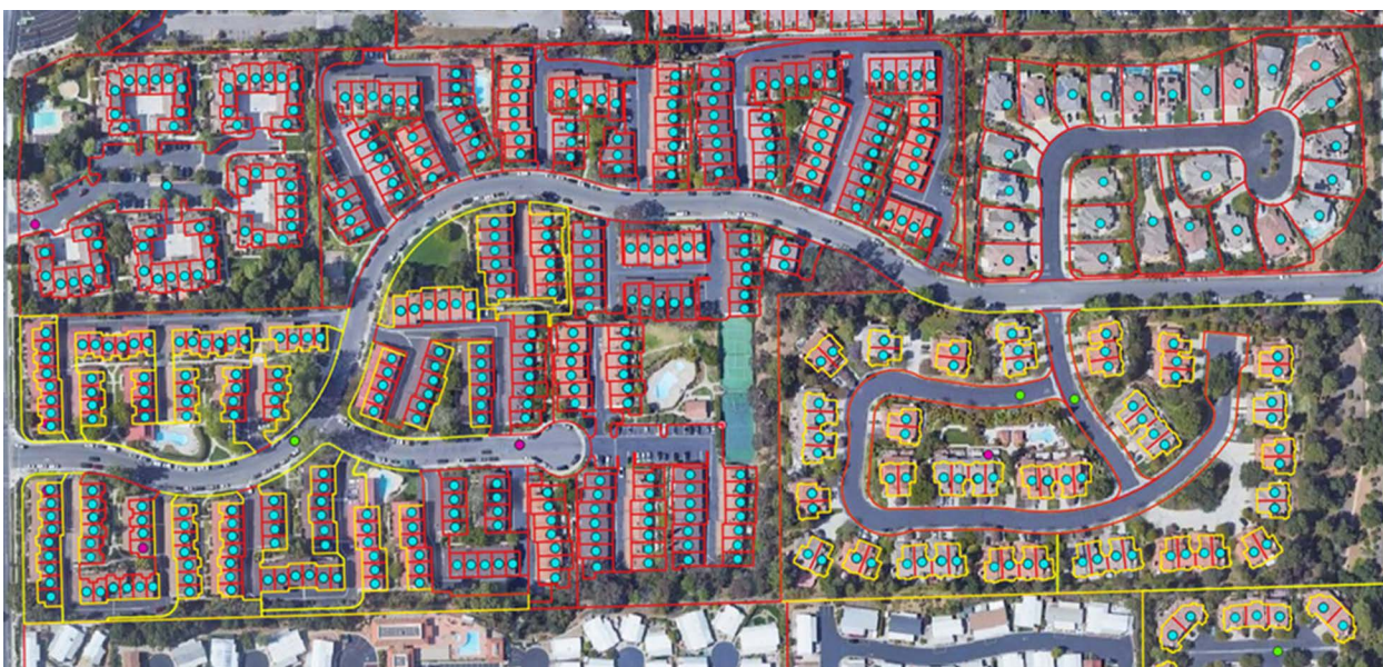
Figure 6. Example of an HOA aerial orthophoto with parcel boundaries (red) and geocoded customer locations (light blue) overlaid within GIS software. DIMs are shown as bright blue/green points, and the parcels irrigated by the DIMs are shown outlined in yellow.
